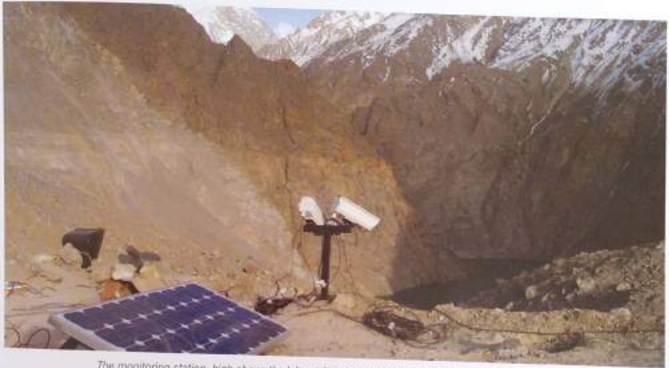
The monitoring station, high above the lake at Attaabad, keeping a watchful eye on the water level
